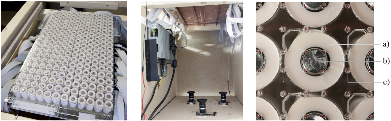
Figure 2: Hardware setup. Left: Array of 228 electromagnets assembled from three modules. Middle: Cameras beneath the table capture the grid of fiber optic cables. Right: Alignment of fiber optic cables. a) Coil bobbin. b) Magnetic core. c) Fiber optic cable.
