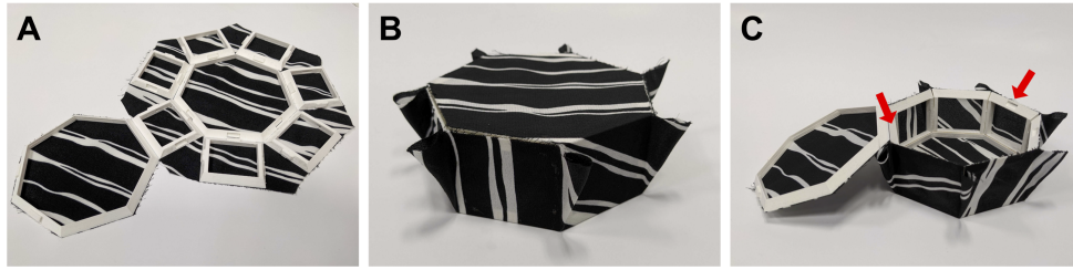
Figure 4: A jewelry case with a lid that can be opened, and with fabric folds as aesthetic elements: (A) The unfolded case with the additional fabric. (B) The closed case and its aesthetics. (C) The case with the lid open; red arrows mark the hinge without connectors and the connector that helps hold the lid closed.
