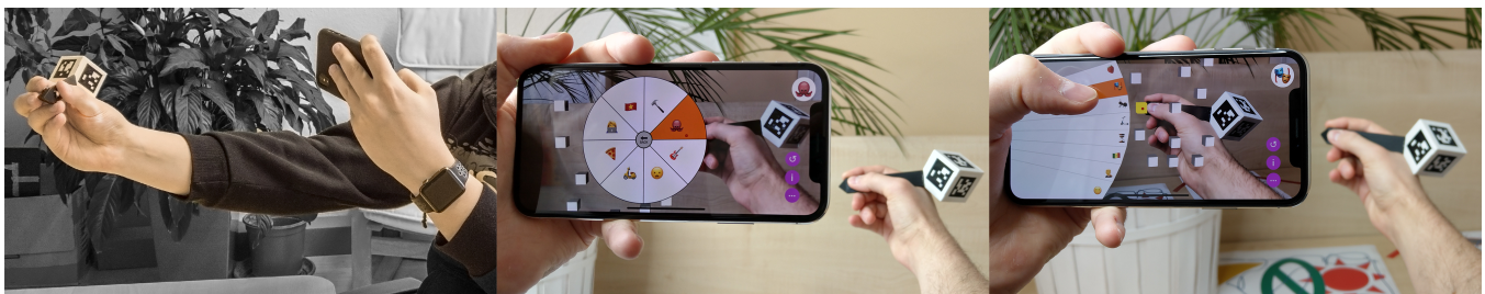
Figure 1: Handheld AR systems with a mid-air pointing device let users interact in Augmented Reality requiring only a smartphone and a custom printed pen (left). We implemented and evaluated menu techniques that use different methods for the interaction with the system, for example, using the mid-air pen (middle) or the hand holding the smartphone (right).
