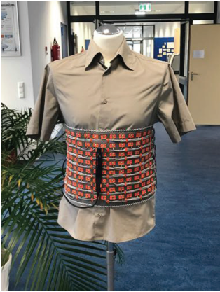
Figure 1: A belt with 16*8 vibration motors and a depth camera on the front side
