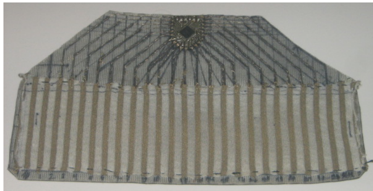
Figure 3.3: The first version—A PCB with an Atmega is connected with the pinstripe textile with conductive thread.
