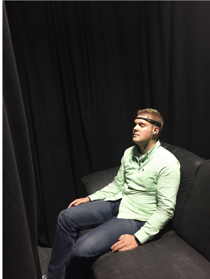
Figure 6.1: Study setup of the Subject-Independent study. Participant sitting on the couch enclosed with curtains, wearing the Interaxon MUSE headband and noise cancelling headphones.
