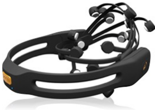
Figure 1.3: Emotiv Epoc 1 , a non-invasive BCI headband with 14 electrodes for signal acquisition.
