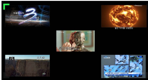
Figure 2.3: Interface for channel selection on TV Screen [Kim et al., 2013]. Green cursor on the top left corner of each channel icon flashes to invoke a response from the user.
