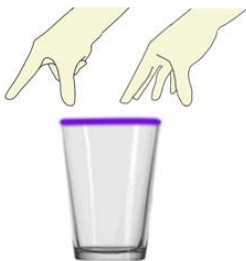
C. Grasp the glass from the top with 2 fingers for fine navigation, and grasp it with 5 fingers for coarse navigation
