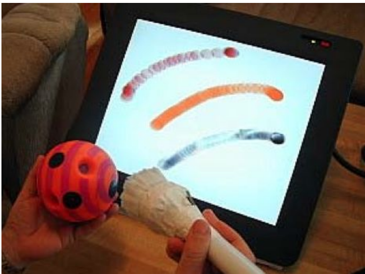
Figure 2.5: I/O Brush allows users to "pick up" different properties of an object, such as color, texture or movement and apply it on the canvas.
