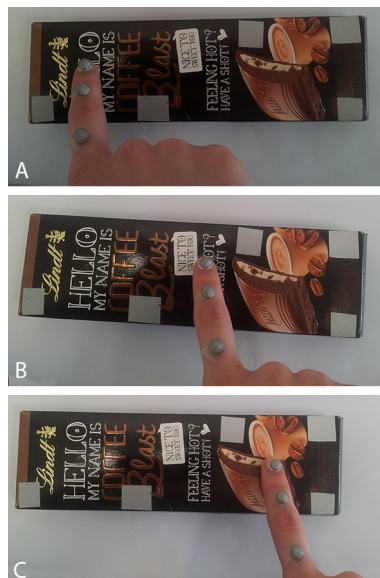
Figure 5.3: Three touch-sensitive areas were defined on the chocolate bar object and were available for mappings.
