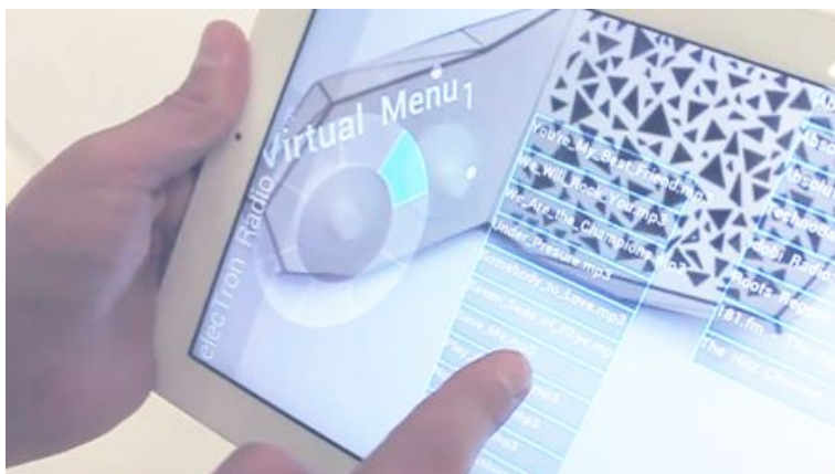
Figure 2.8: Smarter Objects: modifying the behavior of a physical object with an AR application. A user holds an iPad with the AR application in front of the object to identify it, then a respective interface appears on the screen and the user can choose the desired functionality.
