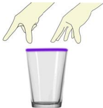
C. Grasp the glass from the top with 2 fingers for volume control, and grasp it with 5 fingers for brightness control
