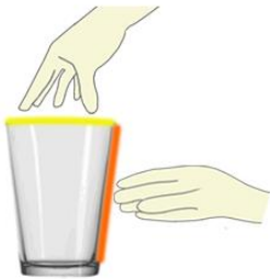
A. Grasp the glass from the top for fine navigation and grasp it from the side for coarse navigation
