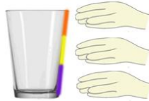
B. Grasp the glass from the top side for volume control, grasp it from the middle side for brightness control, and from the bottom side for video navigation
