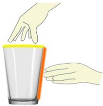
A. Grasp the glass from the top for volume control, and grasp it from the side for brightness control
