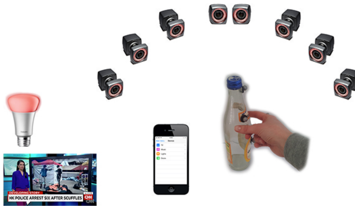
Figure 6.1: The setup included eight Vicor Bonita cameras, objects with reflective markers, iPhone applications for the PBD and GUI approaches, TV application and Phillips Hue smart lights. User's hand was also augmented with three reflective markers.
