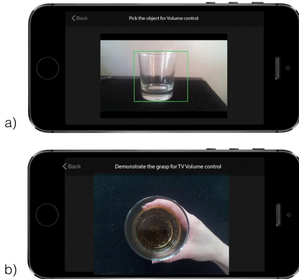
Figure 3.3: Using an object without visible state indicators, such as a glass: a) a user, first, selects an object, and then, b) demonstrates the grasp we would like to map to the selected controller without indicating object positions for the minimum and maximum values.
