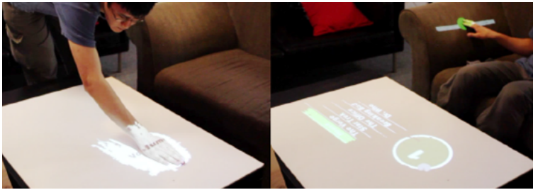
Figure 2.1: WorldKit system: a user performs a swipe gesture on a table or couch surface and instantiates interactors for controlling devices in the living room.
