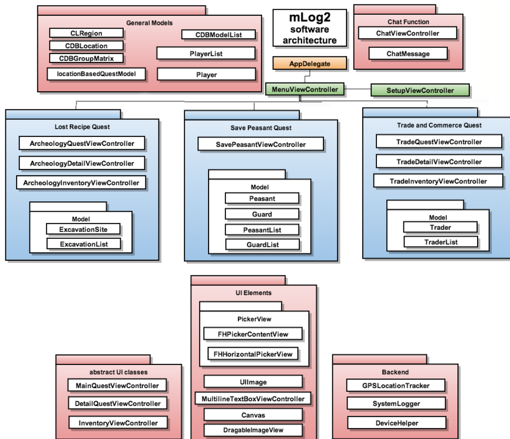
Figure 5.12: Overview of the Software Architecture
