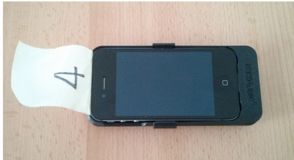
Figure 7.2: Battery pack for iPhone
