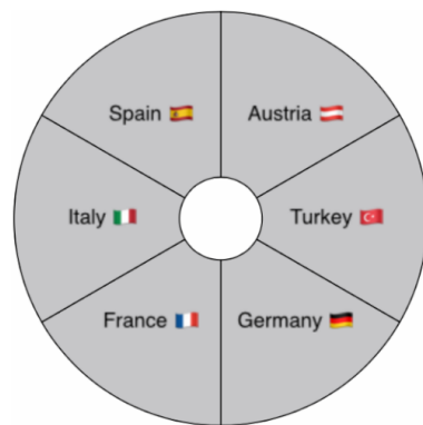
Figure 3.13: Pie menu adaption with six items, opened in the middle above the menu button which is covered thereby.
