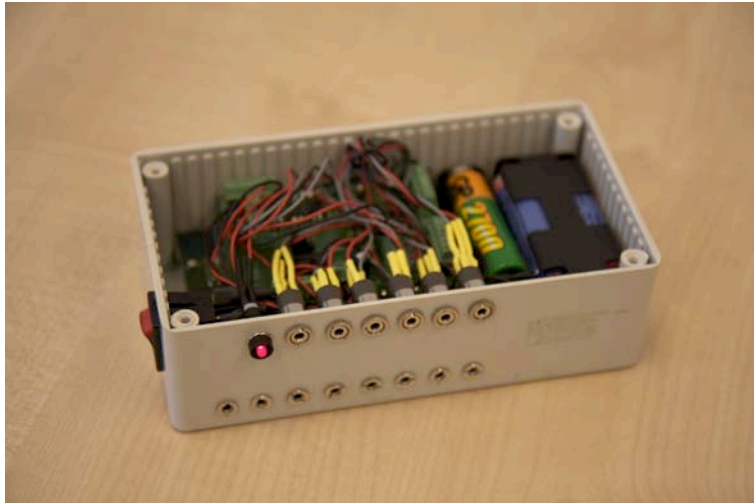
Figure 3.3: First Hardware Prototyp
