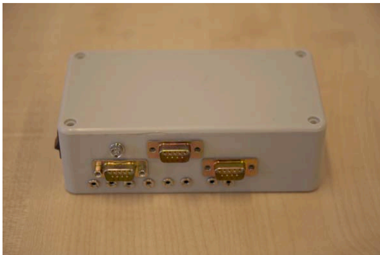
Figure 3.5: Second Hardware Prototype: First version with only six sensor connectors.
