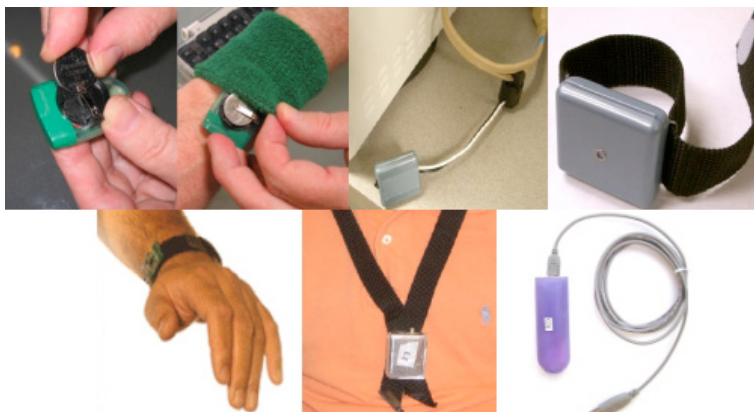
Figure 2.7: A subset of sensors of the wireless sensing kit provided by Tapia et al. [2006].
