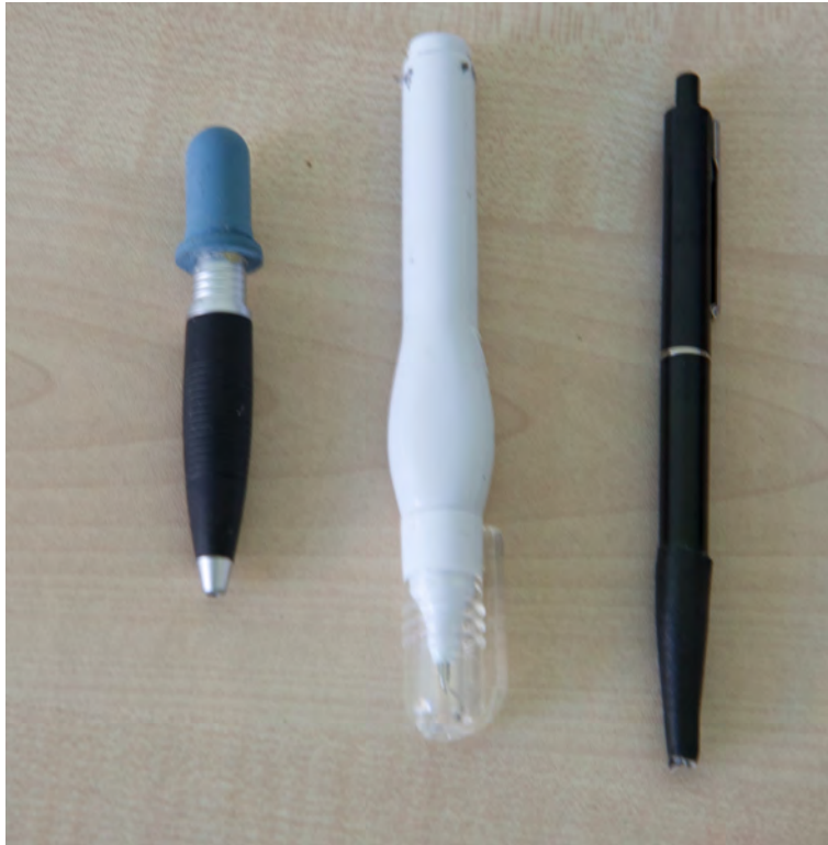
Figure 4.3: Non-Functional prototypes of the pipette concept. On the left side: a small pipette with bulb at the end. In the middle: Pen with the bulb in the first half of the pen. On the right side: classical non-bulb pipette.
