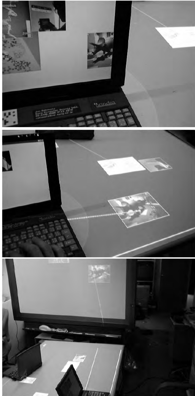
Figure 2.5: An example for hyperdragging: The user drags a picture to the edge of his display (first picture) onto the tabletop (second picture). From this position he drags it onto the wall sized display to present it (third picture). Taken from Rekimoto and Saitoh [1999].
