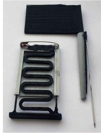
Figure 4.3: Spring and flag with safety pins molten to the conductive part of the brooch
