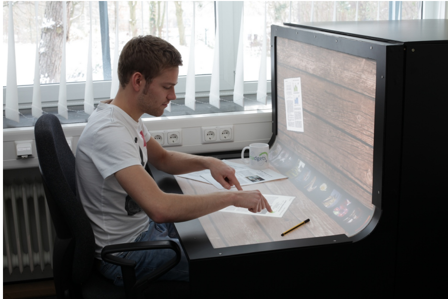
Fig. 6. BendDesk [1] was created according to the most comfortable height for users sitting at it.
