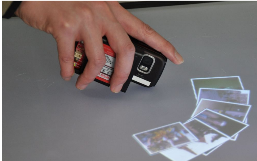
Fig. 15. PhoneTouch connects a tabletop with a cell phone. Courtesy by Schmidt et al. [3].
