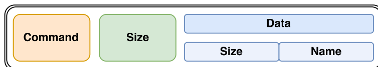
Figure 6.4: The whole protocol header
