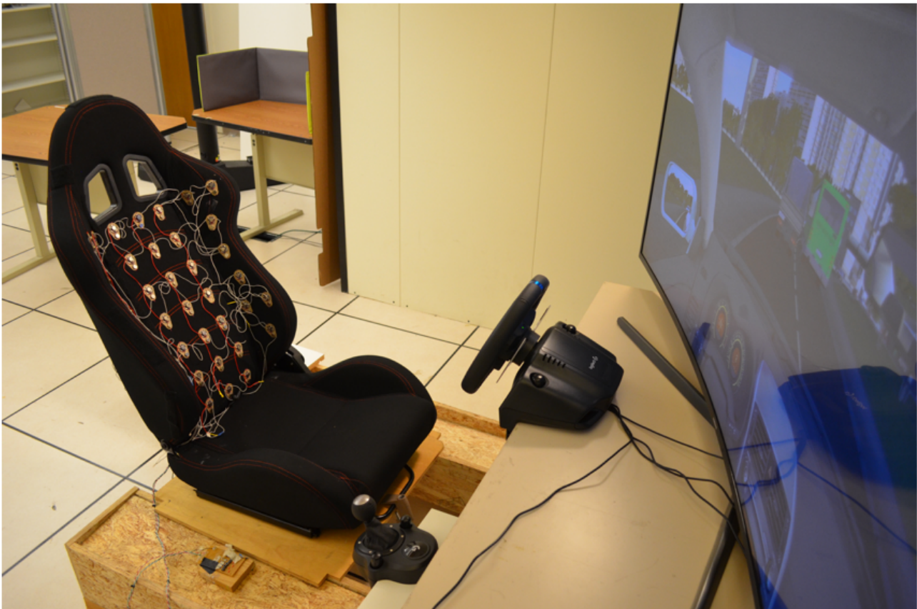
Figure 1. Vibrotactile prototype with a matrix of vibration motors in a car driving simulator setup.
