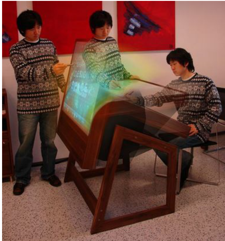
Figure 2.1: The FLUX system that has one tiltable screen surface [Leitner et al., 2009].
