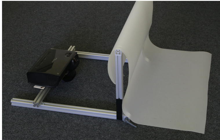
Figure 3.8: Projector prototype that allowed testing of the minimum projection distances, general mounting and how much force is needed to move the frame.
