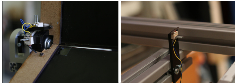
Figure 4.13: The end switches that allow for basic tracking of the screen position.
