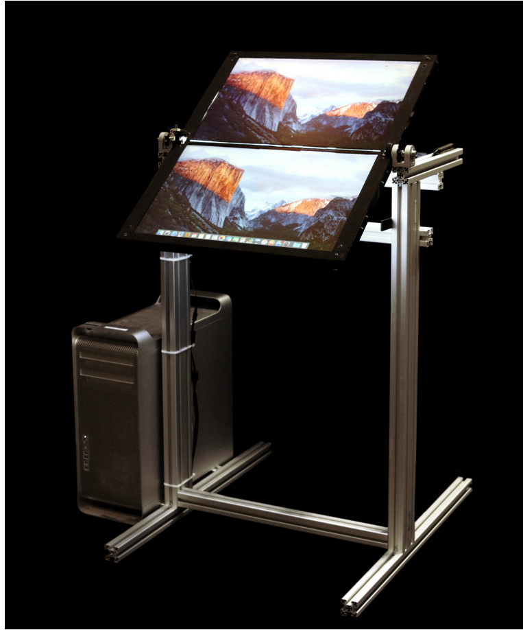
Figure 1.2: Flowdesk is a screen system with two independently movable screens that can adapt dynamically on the users task.
