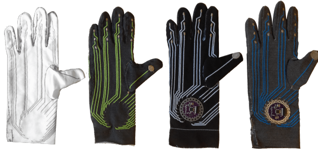
Figure 5.12: Smart-Gloves: iteration refinement with embroidered touch buttons.
