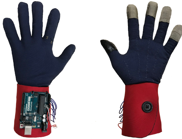
Figure 3.9: Our first prototype includes pressure sensors and a bend sensor
