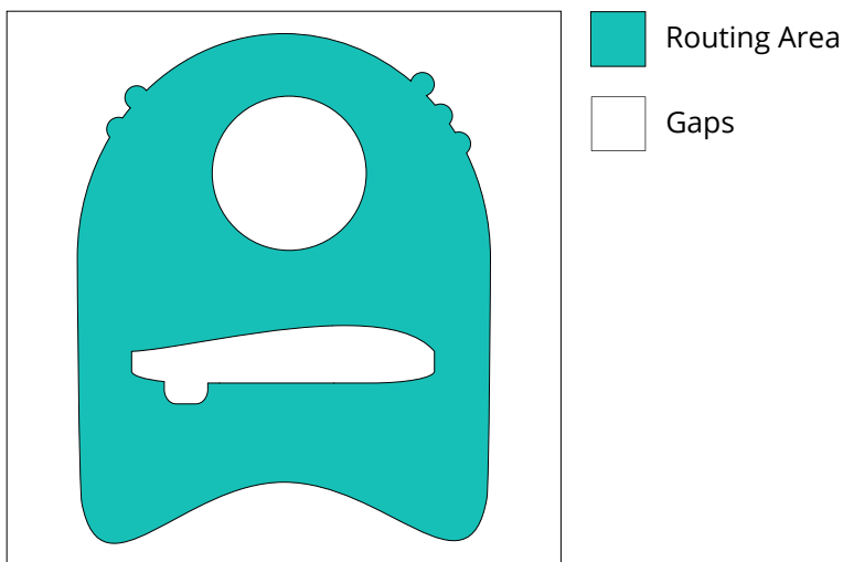
Figure 4.3: Input Pattern: The green area is where the auto-routing takes place. The transparent areas are denominated gaps and excluded when performing the auto-routing.
