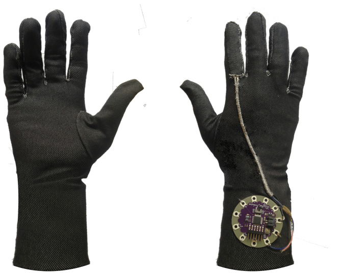
Figure 3.11: Smart-Glove prototype with a flex sensor
