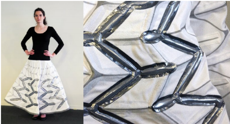
Figure 2.5: Prototyped version of a skirt with an inserted origami pattern of pneumatic actuators, Perovich et al. [2013].
