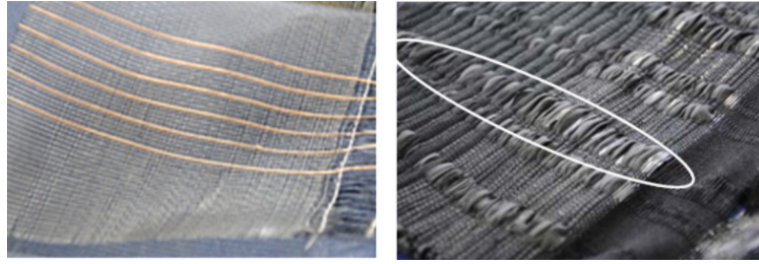
Figure 2.4: Electroactive polymers integrated inside the fabrics, Maziz et al. [2017].
