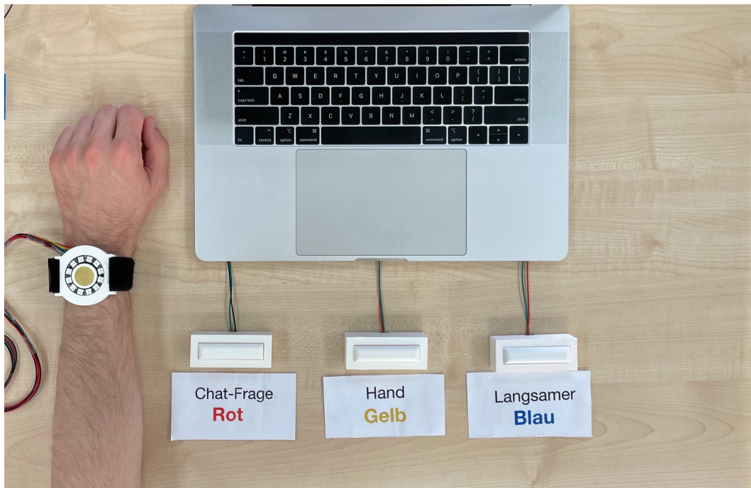
Figure 4.3: Top view of the participant’s desk. Performing the task, participants had to press the buttons when the signal was recognized.
