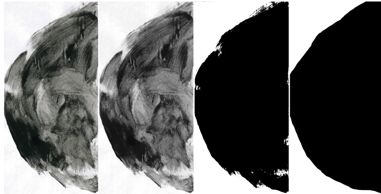
Figure 4.5: Editing process of the captured functional areas of the user study. From left to right: (1) Raw image. (2) Converted to greyscale. (3) Threshold algorithm marking a pixel either black or white. (4) filling of holes after the threshold algorithm.
