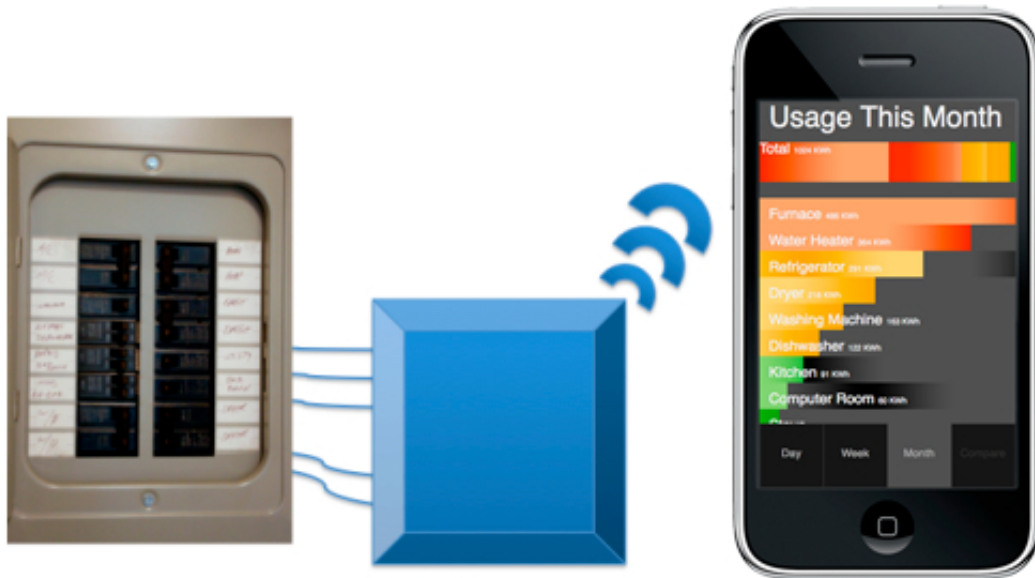
Figure 2.3: Wattbot - Technical Structure and iOS App
