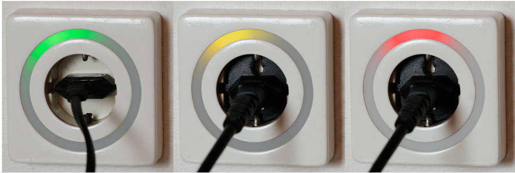
Figure 6.3: Visualization Unit: Rotation Integrated into Self Made Wall Socket ( Low, Mid, and High Energy Consumption)
