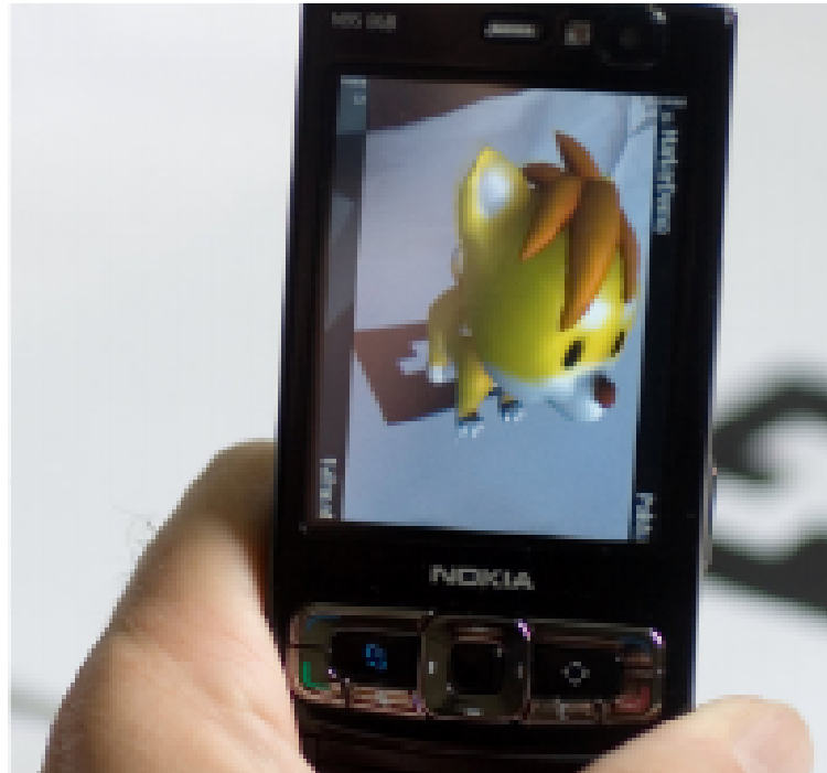
Figure 3.4: Harviainen et al. [2009] used only camera-based input for their application. Even with earlier technology, device motion as a technique was appreciated by users.
