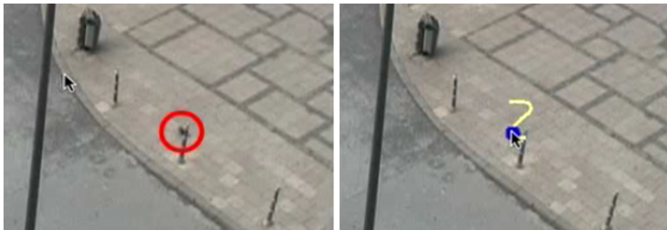
Figure 4.21: Optical-flow-based tracking of small objects in videos. The pigeon covers less than 30 pixels in total (left); still, the optical flow field describes its motion very precisely (right). Faster but less dense tracking methods have problems in such cases—the pigeon, for example, does not contain a single SIFT feature.
