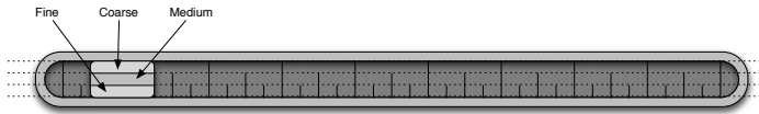
Figure 4.5: Position interface of the Alphaslider by Ahlberg et al. [1994]. Different click targets on the slider thumb explicitly select different control granularities.
