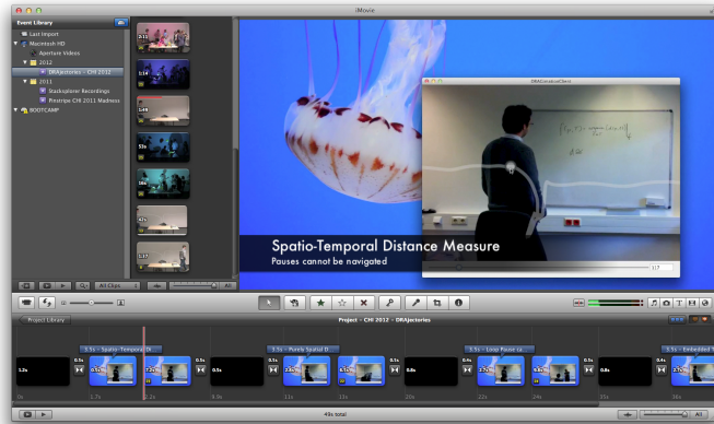
Figure 4.1: Apple's iMovie is a modern non-linear video editing software package. Individual shots or scenes of a longer video clip can be accessed directly, and markers can be assigned to special points in time. Navigation inside a single scene, however, still relies on a scrubbing technique using the playhead in the timeline.
