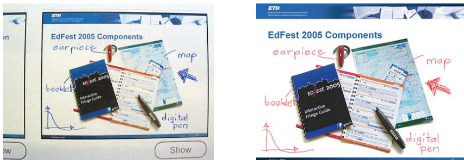
Figure 5.6: PaperPoint slide proxy (left) and digital projection (right). The slide deck can be navigated by tapping each slide’s individual show button with a digital pen. Also, annotations made on the paper version of the slide propagate directly to the digital projection. Source: [Signer and Norrie, 2007]
