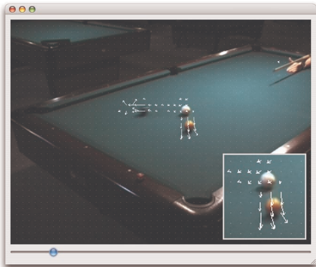
Figure 2. The flow field (shown in white) stores the pixel correspondences between pairs of adjacent frames. These correspondences allow us to recreate the movement trajectories of arbitrary objects in a scene, such as the billiard balls in this table shot.
