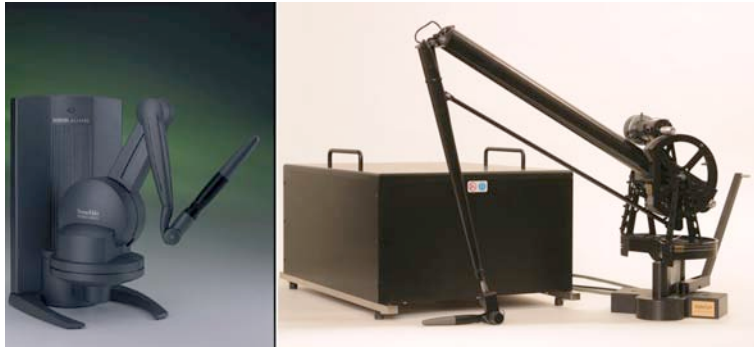
Figure 2.7: Two haptic devices from the Phantom series by SensAble Technologies - a Phantom Desktop device on the left and large Phantom Premium device on the right; photos from SensAble Technologies
