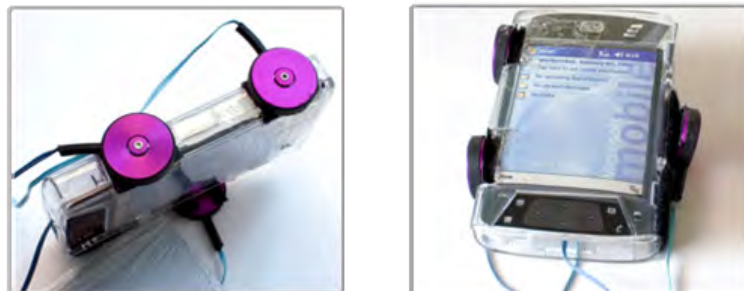
Figure 3.12: Multi-actuator PDA as proposed by Hoggan et al. [2007]
