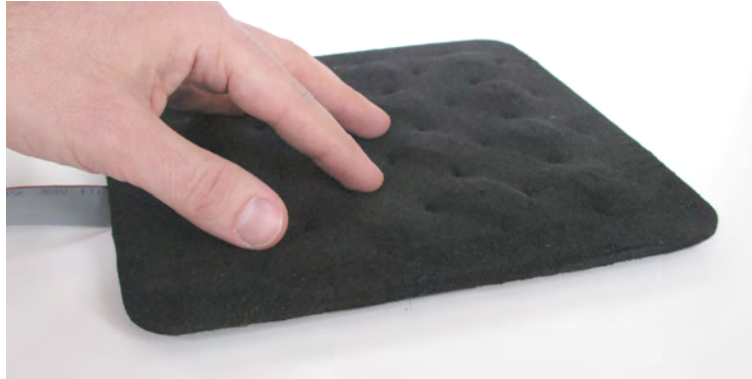
Figure 3.8: BubbleWrap haptic display prototype (Bau et al. [2009]).
