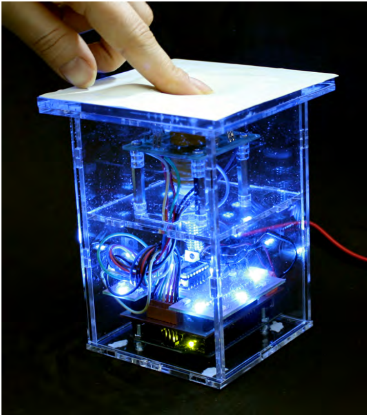
Figure 4.7: The second prototype is a fully functional travel version and simulates one button to demonstrate the possible feedback modes.
