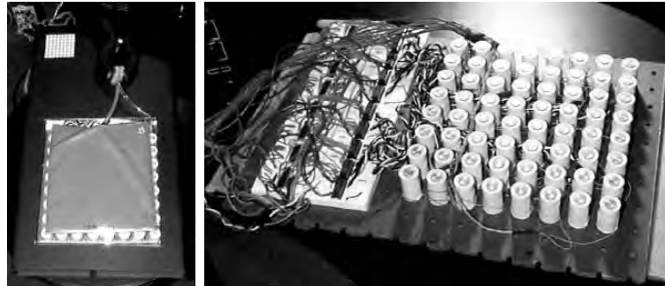
Figure 3.14: The liquid haptic output pad by White [1998]. Left: final prototype with liquid filled bladder on top. Right: the underlying array of electromagnets without the bladder.
