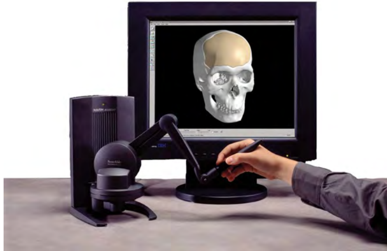
Figure 3.6: The SenseAble Phantom force-feedback device depicted in a 3-D modeling scenario (Massie and Salisbury [1994]).
