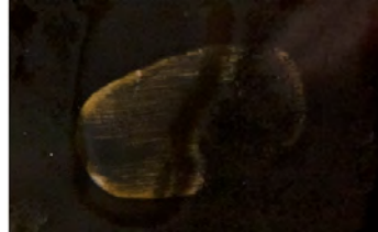
Figure 4.6: A touch from a finger on a MudPad overlay as it is seen from below. The particles directly underneath the finger do not get displaced completely.
