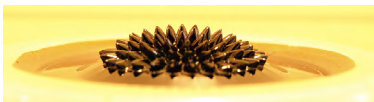
Figure 1.1: Ferrofluid exposed to a magnetic field showing spikes in direction of the magnetic flux lines.
