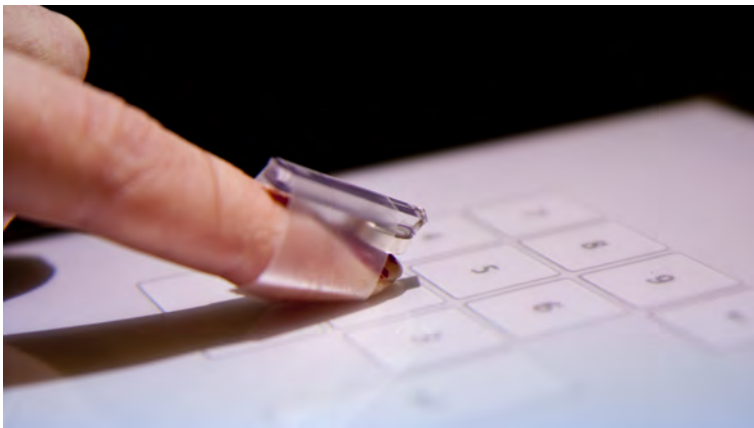
Figure 6.3: Nail-mounted permanent magnet for tactile feedback without the MudPad overlay.
