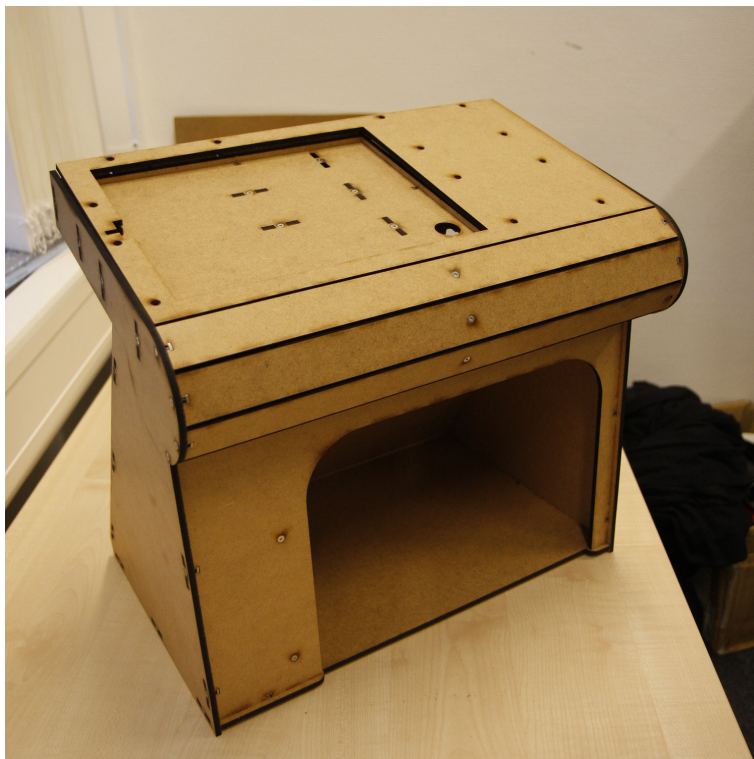
Figure 5.5: Photo kiosk right after assembly (without the door and the foam rubber).
