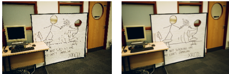
Figure 4.7: Comparison of resizing image of 1024×680 pixels to 300×200 pixels: Automatic resizing from UIImageView (left); Resizing with CGContextSetInterpolationQuality method using kCGInterpolationHigh parameter in Quartz 2D (right).
