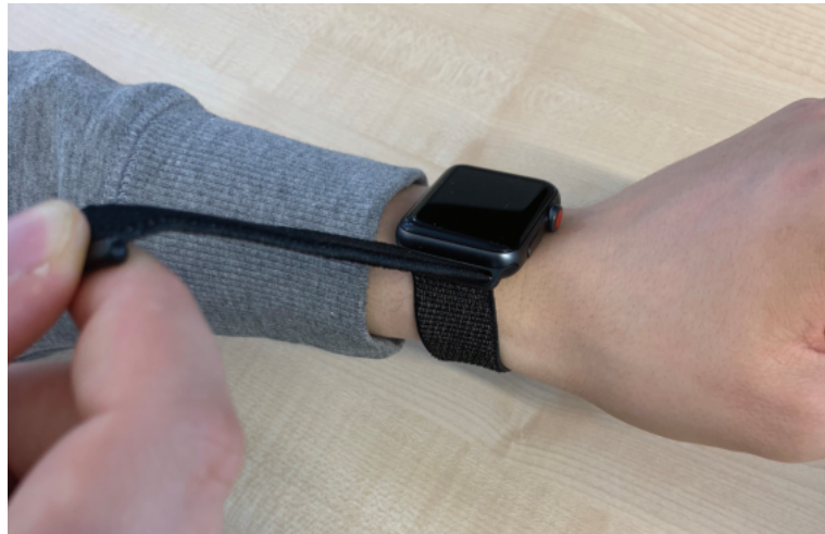
Figure 7.1: The Hook-and-loop band design taken from Apple watch sport band design. This design makes it easy for the band to fit most wrist sizes, keeping an affordance for pulling at the bottom of the band.
