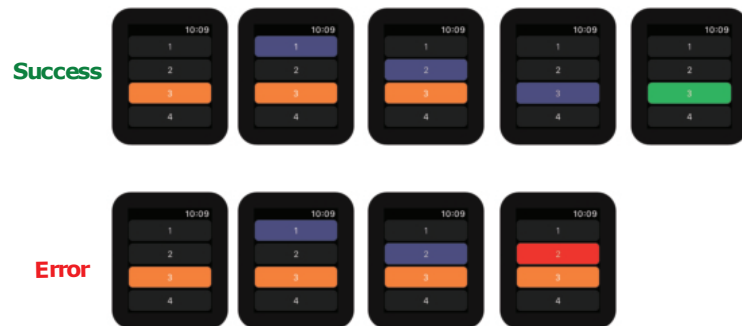
Figure 8.2: Visual Exploratory Watch App with a menu selection task. The user navigate through the menu in order to select the highlighted target in orange. In the success scenario at the top, the user select the right target. In the scenario at the bottom, the user selects a wrong menu item.
