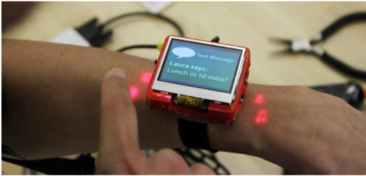
Figure 4.4: Skin Buttons [Laput et al., 2014]. User selects the projected icons on the skin by pushing his finger on them.
