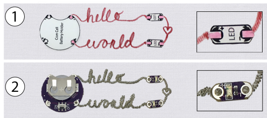
Figure 3. 1. Component Stickers represent electrical components in a hand-sketch circuit. Pin grooves designed to enlarge component contact area. 2. Stickers replaced with hardware counterparts after embroidery.
