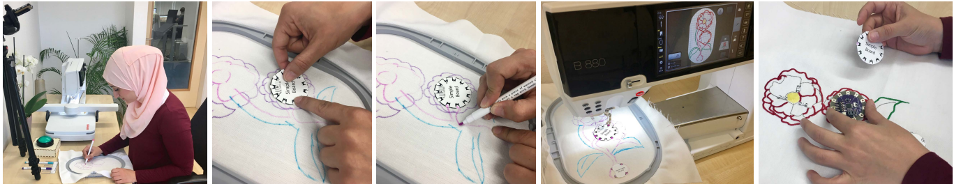
Figure 1. Sketch&Stitch workflow: 1. The user sketches an artwork directly on the fabric, 2. she uses Circuitry Stickers to plan the circuit layout, 3. she draws circuit traces to connect the stickers, 4. the system takes a picture of the sketch, converts it to embroidery patterns, and sends them to an embroidery machine for stitching using conductive and non-conductive threads, 5. the user replaces Circuitry Stickers with real electrical components and attaches them to the fabric.
