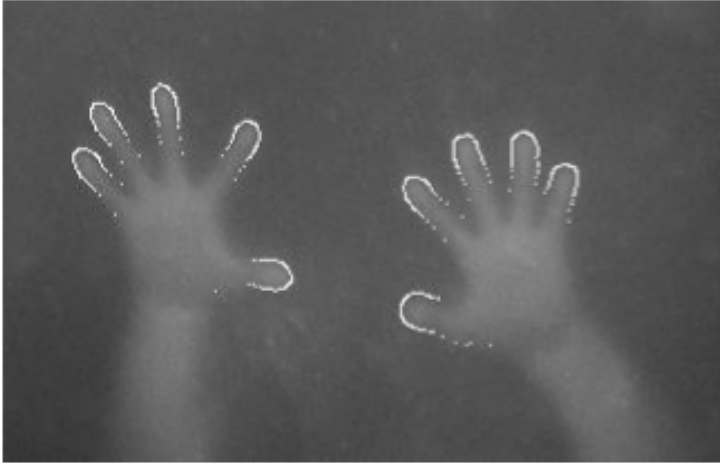
Figure 2.11: Finger Contours determine the symmetrical lines around each finger and use them to compute the finger orientation [Dang and André, 2011].
