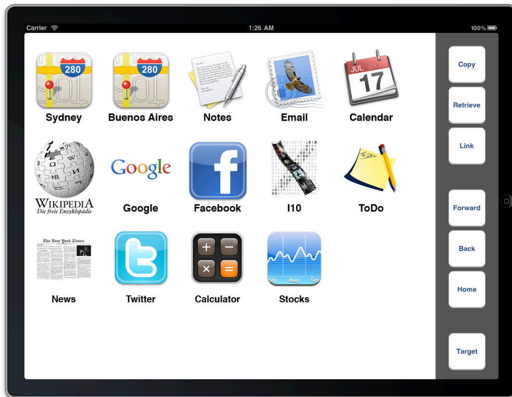
Figure 4.6: The Tangible Windows prototype shows a bar next to any task applications that is used to trigger multi-device operations.
