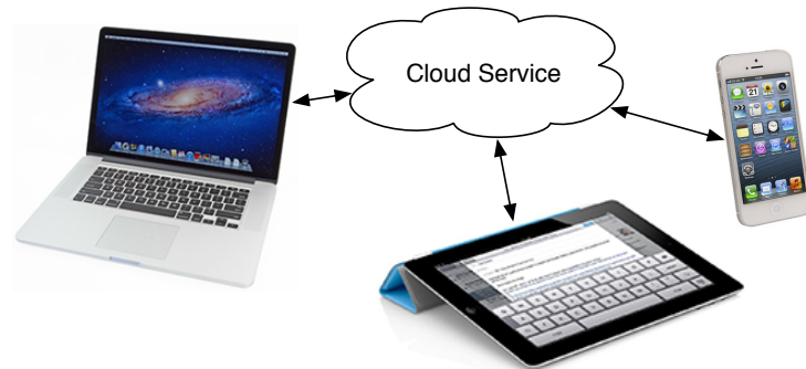
Figure 1.2: Cloud sharing services synchronize local copies of digital content by propagating changes between all connected devices “through the cloud”.
