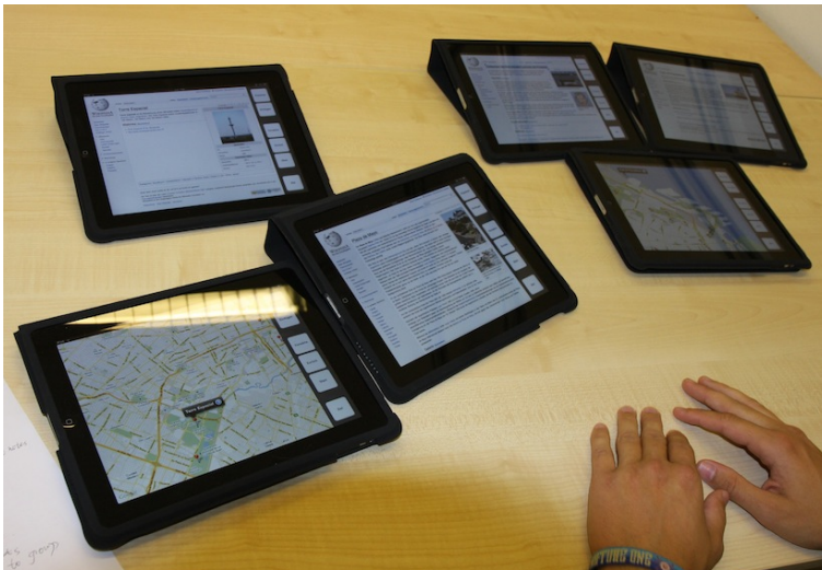
Figure 4.7: An example arrangement of multiple Tangible Windows from the user study. Each group of three devices represents two identified sights: two devices show the Wikipedia articles about the sights, and the third device shows a map that can be switched between the sights via the back and forward operations.
