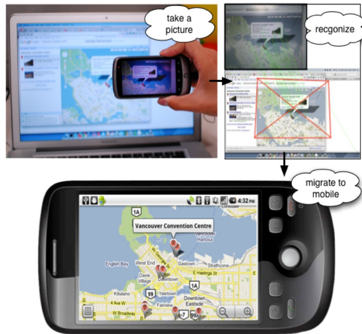
Figure 3.7: Deep Shot allows users to migrate a task between a mobile phone and a desktop computer by taking a picture of the desktop computer's screen with the mobile phone's camera. The task can be migrated to the mobile phone using deep shooting as depicted in the figure, or it can be migrated to the desktop computer using deep posting. Picture taken from Chang and Li [2011].
