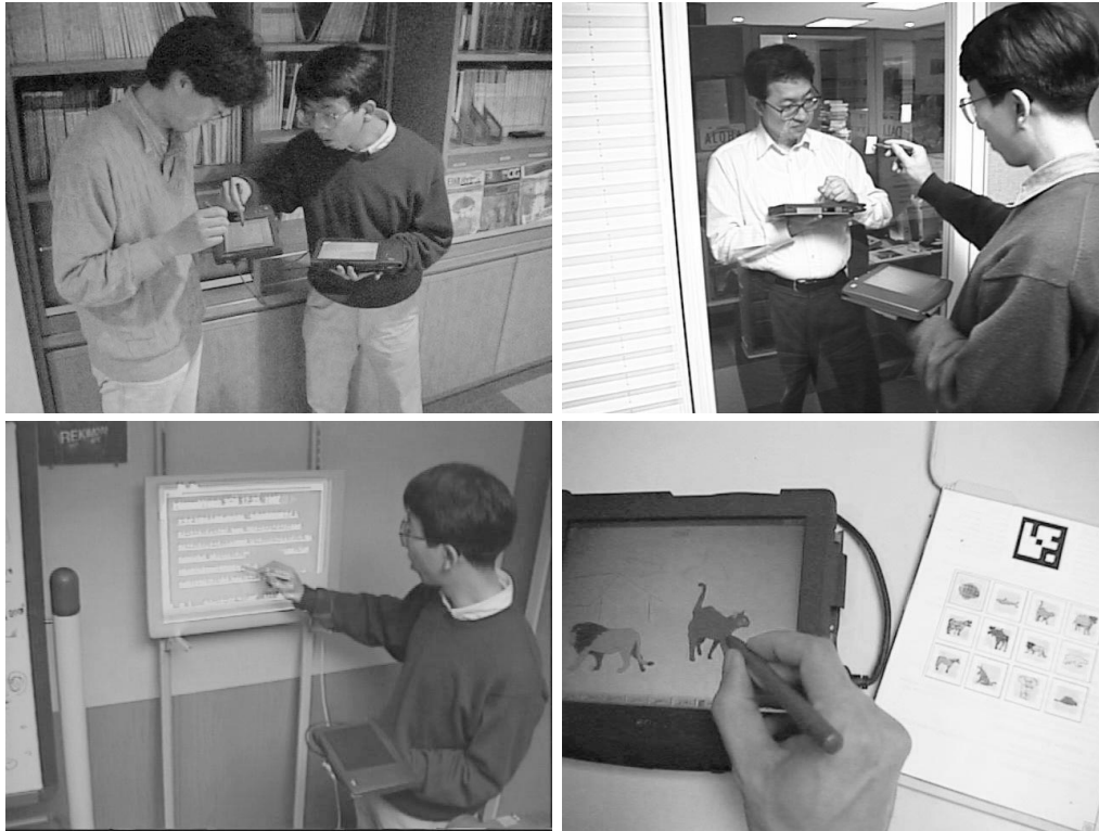
Figure 3.2: Pick-and-drop has various application areas: Users can exchange information between personal tablets (top left) or through a shared display (top right). Interacting with a wall screen can be augmented with a tablet display (bottom left). Objects can be picked up from a printed representation of the object (bottom right). Pictures taken from Rekimoto [1997].
