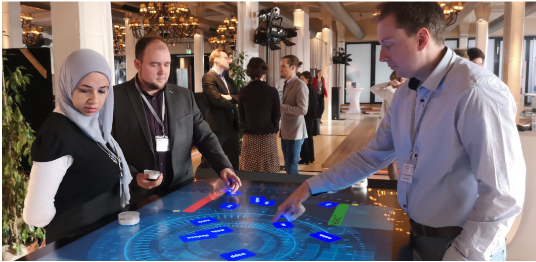
Figure 2.13: A TABULA learning application as presented during the Informationstour Erfahrbares Lernen a by the German BMBF. Here, TABULA tangibles are applied as tools to collect virtual cards into bins. If a card is moved into the wrong bin, the tangible gives subtle feedback via vibration.
