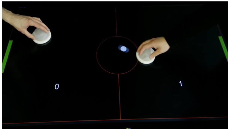
Figure 2.3: A virtual air hockey game with physical mallets. The tangible mallets are detected by the screen and thus can control the action displayed.
