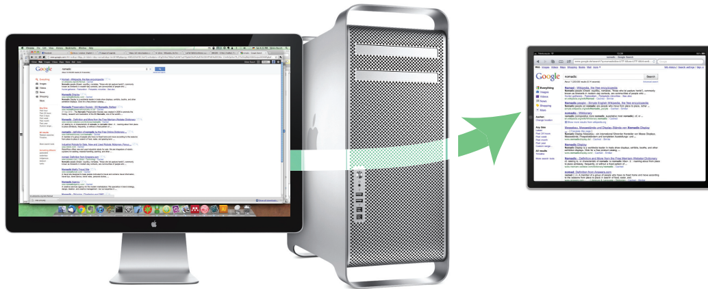
Figure 1.1: Nomadic Applications in action. A browser gets migrated to another device, where it adapts to a device-appropriate form
