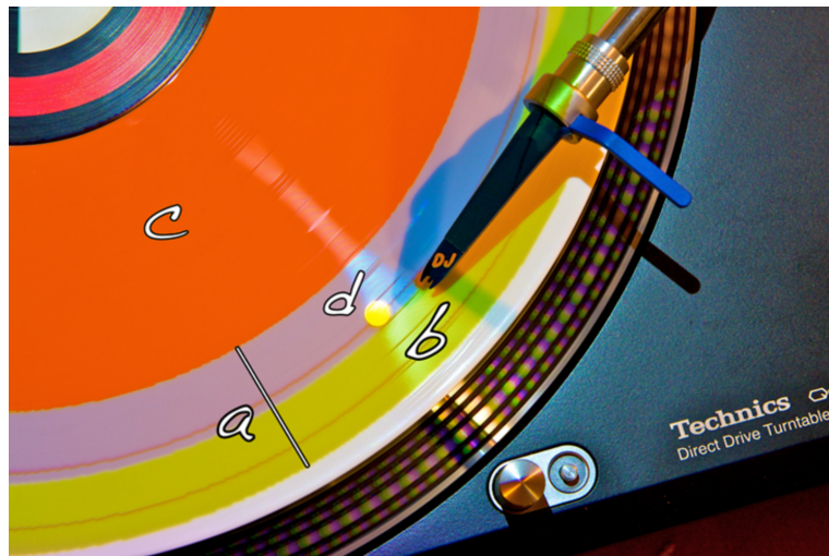
Figure 3.5: DiskPlay feature overview: (a) tracklength on the vinyl - (b) played part of the track - (c) unused part of vinyl - (d) cuepoint
