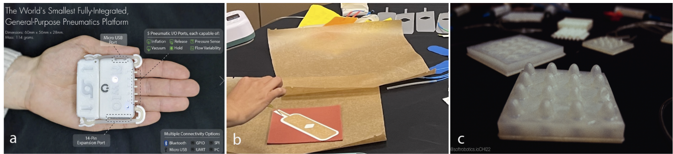
Figure 1: a) FlowIO device that will be introduced to workshop participants; b) Hands-on activities and c) soft robotic prototype demo from the workshop at CHI'22.
