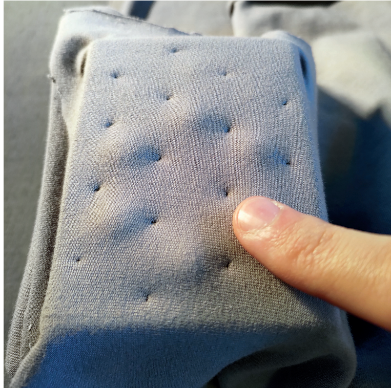
Figure 1.2: The part of our prototype users interact with - the bubblepad. A ring of six cells is currently inflated. A finger presses down on one of the cells.
