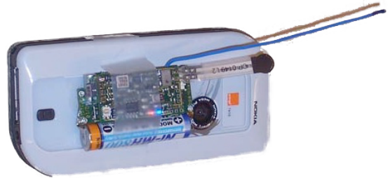
Figure 1. Back view of a mobile phone augmented with a Smart-Its sensor board in iStuff Mobile. The sensors can be attached to the phone in whatever position the designer finds most appropriate. The pictured Smart-It contains a 3D accelerometer, microphone, and sensors for light, pressure, temperature, and voltage.
