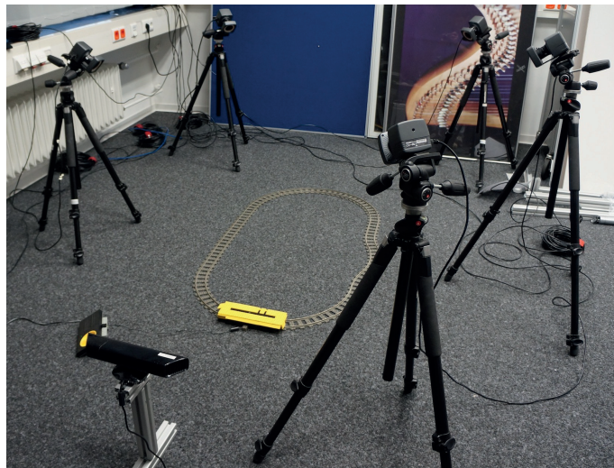
Figure 4.1: Picture of the setup used for evaluating tracking error. Five VICON Bonita cameras are laid around the tracks, shaped as an oval with a small bump. The Kinect depth camera is placed in front of one of the sharp curves of the tracks.
