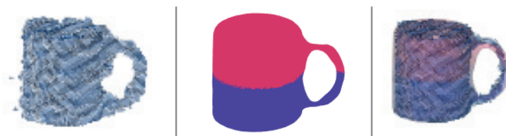
Figure 3.9: Initial pose estimation. The point cloud obtained from the Kinect (left) is used to determine the pose of the loaded model (middle). The result is an estimation of the model on the scene detected by the Kinect (right).
