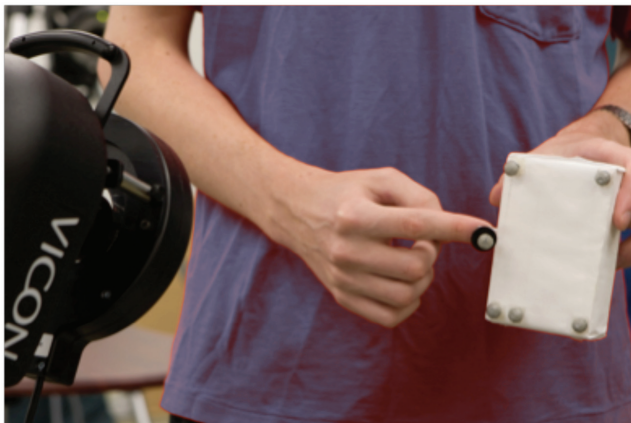
Figure 2.11: DisplayObjects setup, composed by: augmented fingers and objects by VICON markers; and VICON tracking cameras
