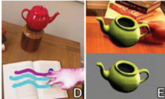
Figure 2.9: An object being tracked (right) and touches being detected (left) by KinectFusion. From [Izadi et al., 2011]
