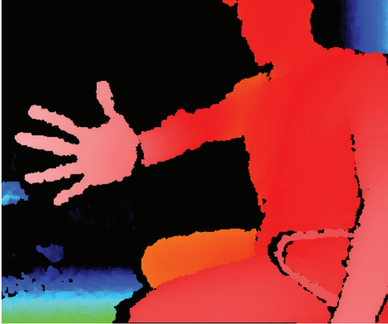
Figure 2.2: Colored depth image of a person obtained using a Kinect. Distances correspond to a color spectrum ranging from light red to dark blue.
